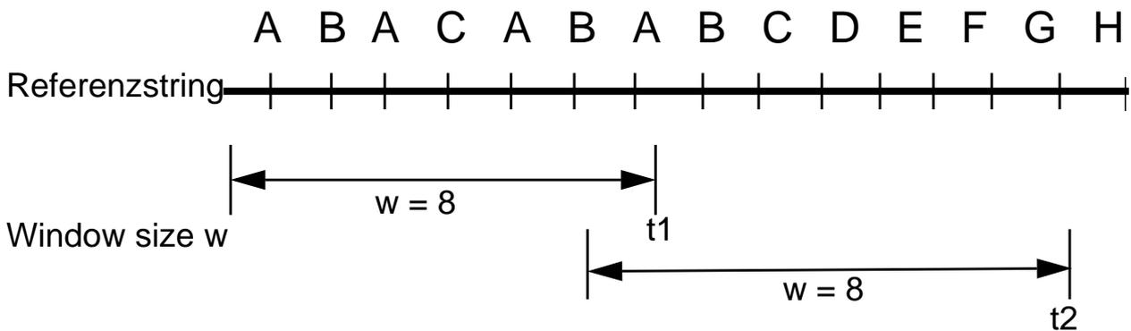
Working set size  $W$                        $W(t_1, w=8) = 3$                        $W(t_2, w=8) = 8$
