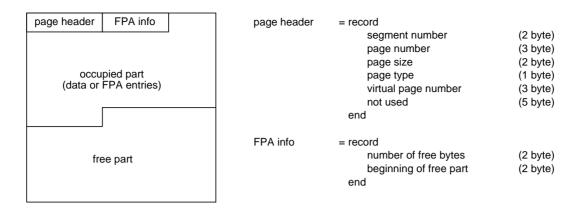
Figure 5: Internal structure of a page
