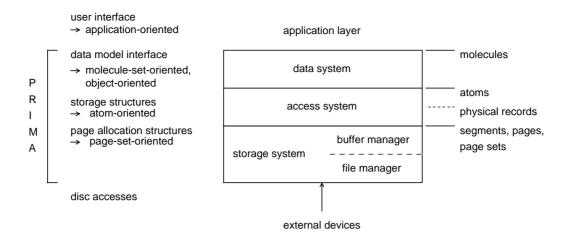
Figure 1: Architecture of a non-standard database system
