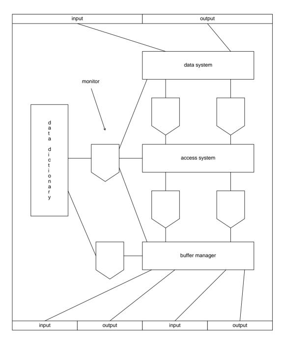
Figure 11: Internal structure of the team type PRIMA
