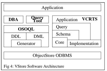
As already mentioned, VStore is implemented on top of *ObjectStore*. In the following we explain the software architecture of our prototype system (see fig 4). A database administrator may use a tool (*DBA*) to install a schema, or to influence *OSOQL* which is the DDL and DML compiler of VStore. A *Query Tool* allows for compiling queries with OSOQL and saving the corresponding code. These
