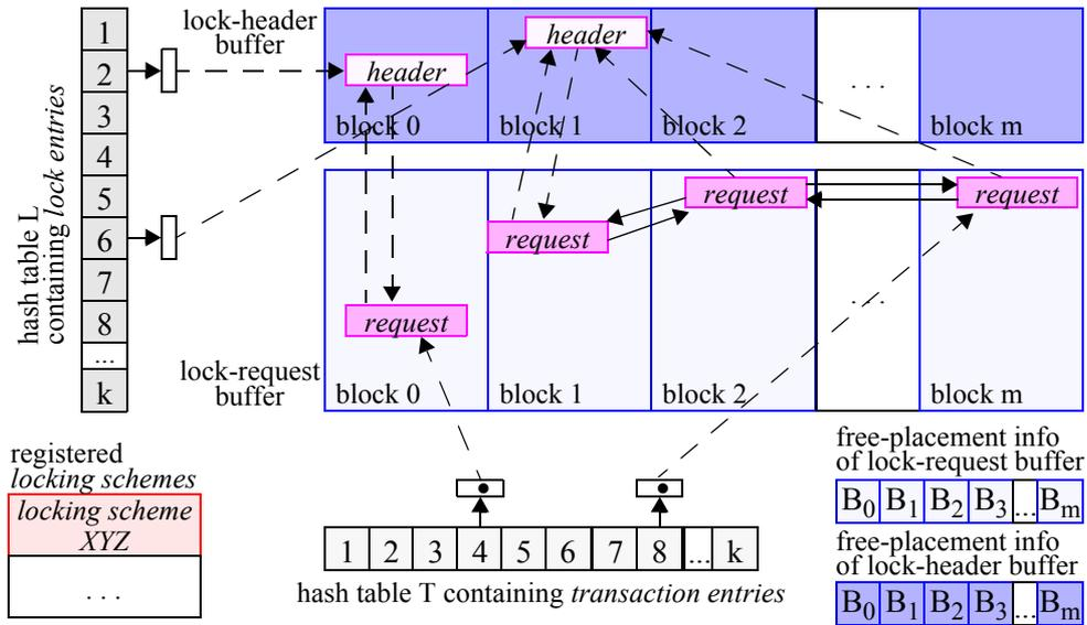
Figure 3. Data structures of a lock buffer
