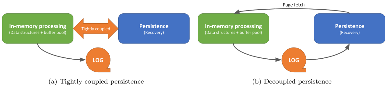
Figure 1: Differences between traditional and proposed architecture.
