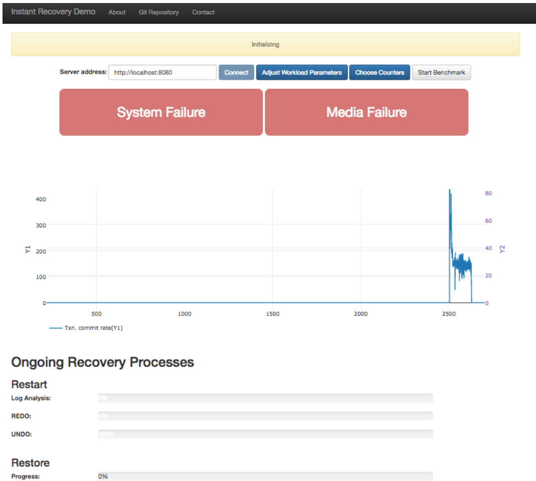
FIGURE 5.1: Loading database and injecting system failure.
