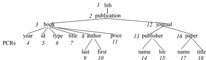
**Figure 7: Path synopsis using PCRs to identify paths to the root**
